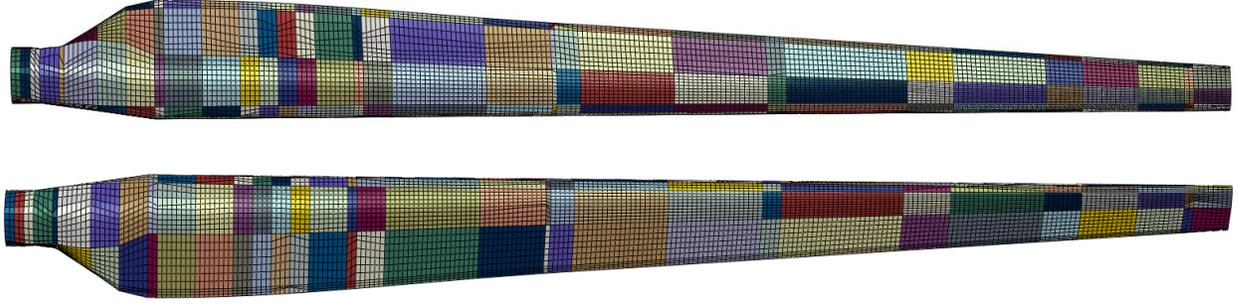
Figure 6.2 Section divisions of the SWiFT wind turbine blade originally defined by the structural finite element model.
