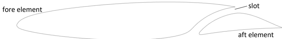
Figure 1.1 Conceptual depiction of the slotted, natural-laminar-flow airfoil design (ref 18).
