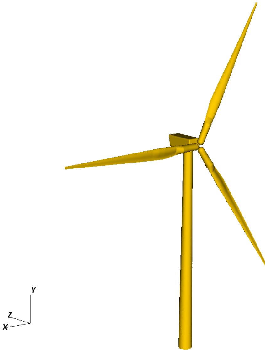
Figure A.1: Horizontal axis wind turbine. The rotor plane diameter of the wind turbine is the diameter of the disk that the blades form when rotating. The height of the wind turbine is given by the height of tower which is the structure that holds the three turbine blades.
