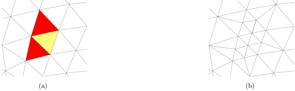
Figure 4.3: Example of h -refinement to eliminate the presence of hanging nodes. (a): Original mesh where the red elements represent elements flagged for regular 1:4 refinement and the yellow element represents a forced 1:4 refinement in this element due to the generation of two additional nodes. (b): The subsequent h -refined mesh.
